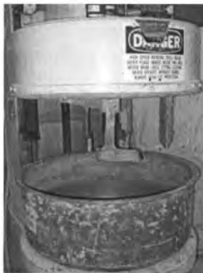
Figure 3.1 Rotating concrete pan mixer
