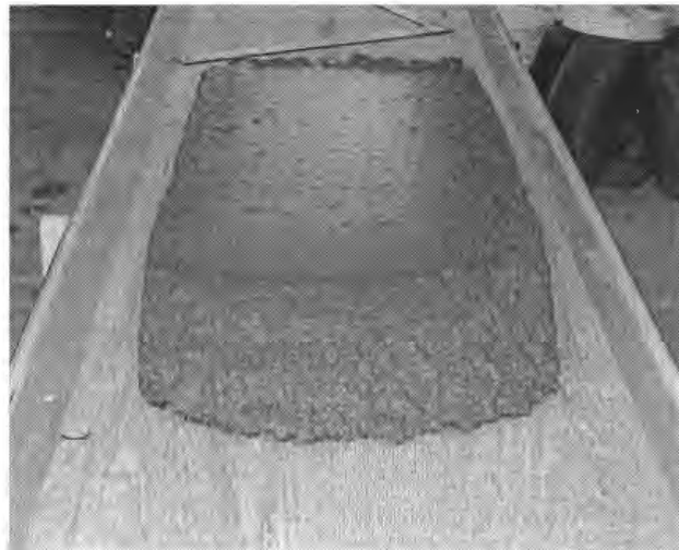
Figure 4.36 Mini-paver test section for SF SCC
