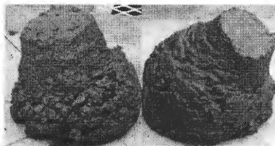
Figure 4.12 Slump test results-poor compacted
